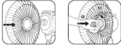
**Step 2** - Install the blade onto the motor shaft by tightening the blade screw.
