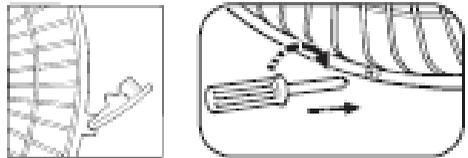
**Step 4** - Tighten the grill locking screw at the bottom of the rear grill.
