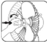
**Step 3** - Centre the front grill by aligning the central logo so it is horizontal and parallel to the floor. Then, secure the front and rear grills completely together by snapping 5x grill clips into place.
